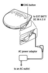
The CD player charges the batteries. The "CHG" indicator turns on in the display, and the indicator sections of [1] light up in succession. When the batteries are completely charged, the "CHG" and [1] indicators turn off.
